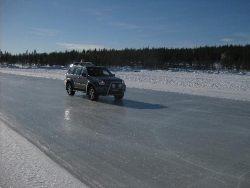
Figure 7. The test on the roughen ice were executed on the ice of the lake. The test on the smooth ice and most of the tests on packed snow were executed on the land track.
