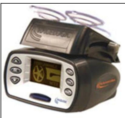
Figure 6. In the picture one of the cheapest models, Performance Box. The small device can be attached for example on the wind screen using suction pads. Also a small GPS antenna is needed. The antenna should be attached outside, on the vehicle roof, with the magnet. The in-vehicle device and the antenna is connected with a wire.
