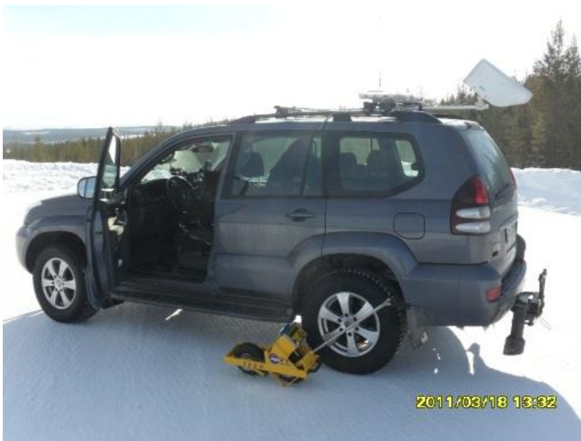
Figure 5. The measuring vehicle in the study. T2GO in front of the vehicle, DSC111 (white box) on the roof and RCM411 in the rear, near the ground.
