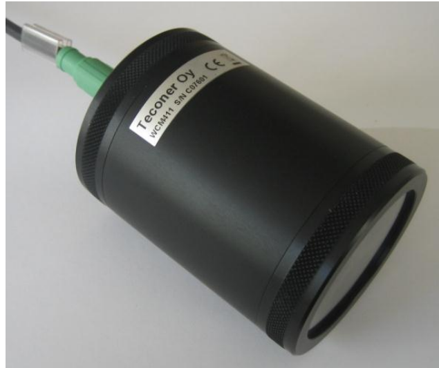
Figure 2 A photograph of Water Content Monitor WCM411. Diameter of the sensor is 75 mm and length 100 mm. The sensor cable is equipped with a 5 lead connector.
