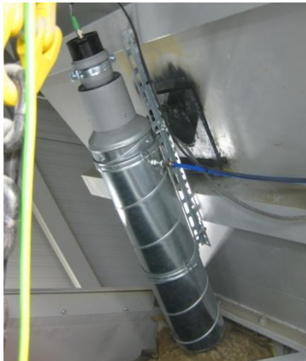
Figure 3 An example of a WCM411 installation over a silo feeder belt with a dust protection tube.
