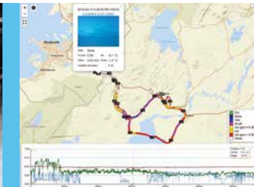
Detected surface states along the driven route on a map interface in Friction Road Map.
