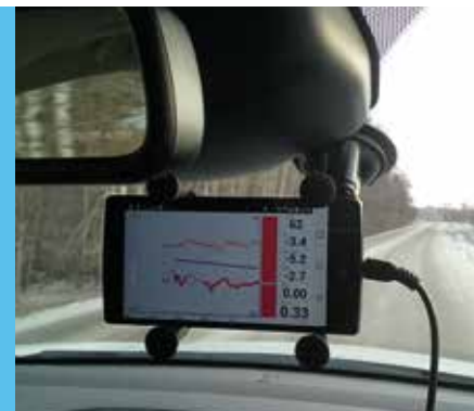
Mobile phone user interface in the vehicle. The system includes a braking friction meter application on the mobile phone.
