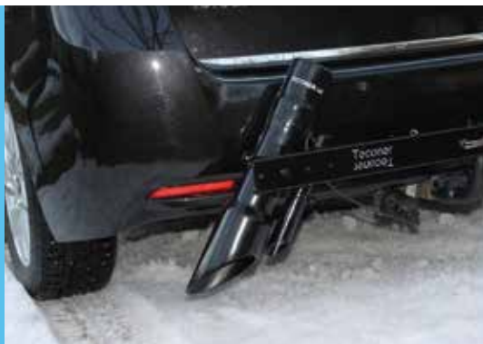
Installation of RCM411 Road Condition Monitor in the vehicle.
